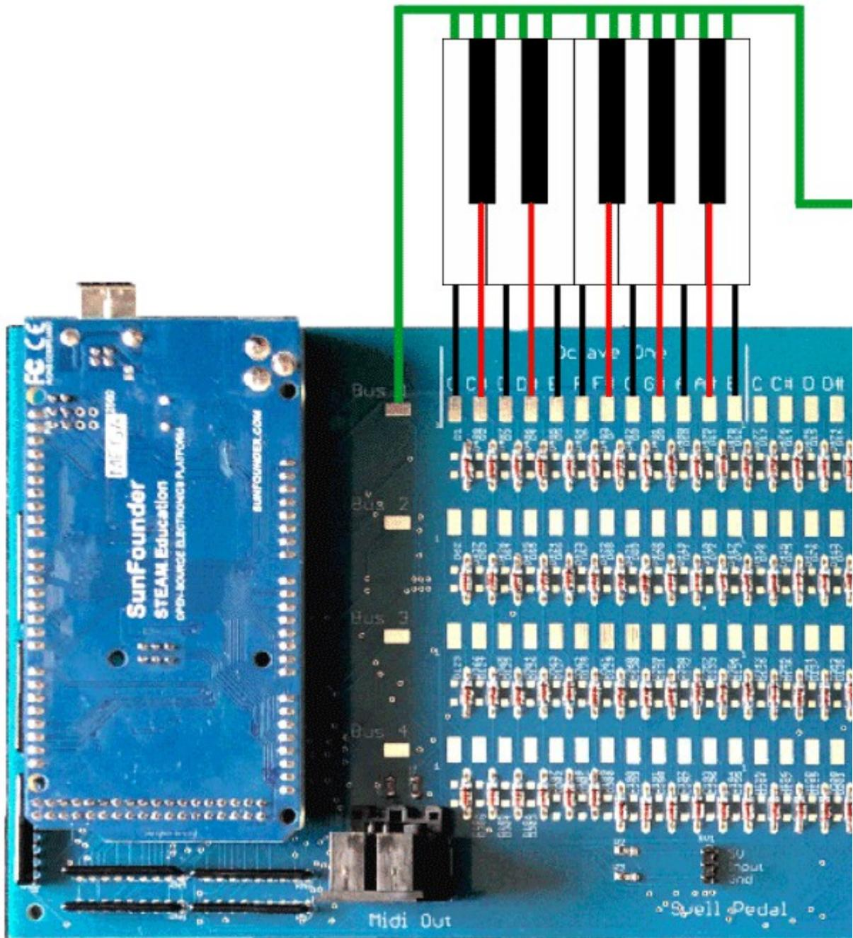
In the picture above I have shown a keyboard connected to the encoder. Only a single octave is shown for clarity, but obviously you would connect all five octaves in this way. However, you are not limited to using just keyboards. You can substitute stops or pistons for the keys in the above picture. So for example, you could connect a keyboard to Bus1 & Bus2, your pedals to Bus3 and your stops and pistons to Bus4.
